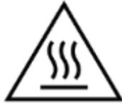
Figure 1.4: This symbol indicates the presence of a hot surface that may cause skin burn.
