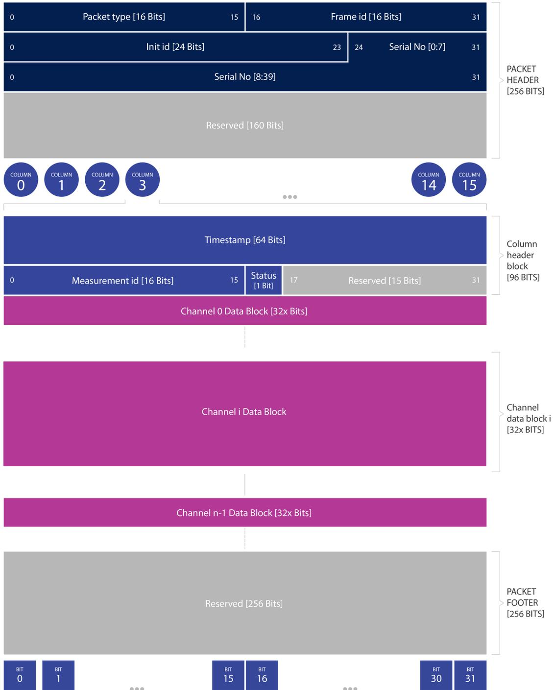
Figure 6.1: Configurable Data Packet Configuration
