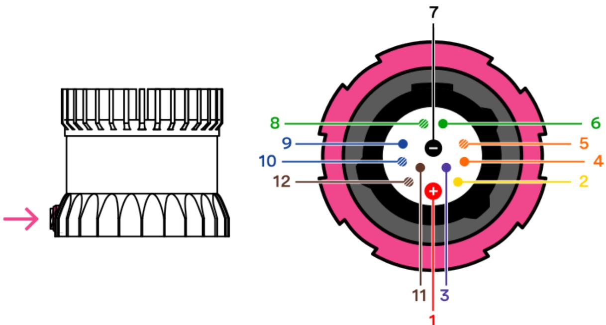
Pinout and wire gauges for Types 1, 2, and 3 (1000BASE-T) cables
