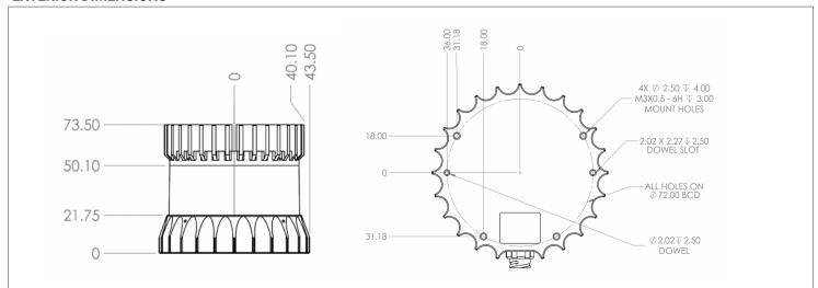
Note: For modular cap design sensors, please refer to the "Radial Cap" and "Flat Cap" CAD models in the "Product Details" section of our website for dimensions
